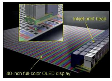
**Figure 3.13.** Schematic representation of inkjet printing for manufacturing of OLED displays. (Digital imageMaker international 2014)
