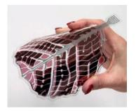
Decorative solar cell can be used to power battery-less sensors for lighting control. (Source: VTT)
