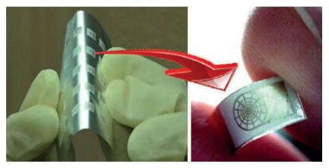
Figure 3.18. Thermocouple sensor. (Source: Wang 2010)
