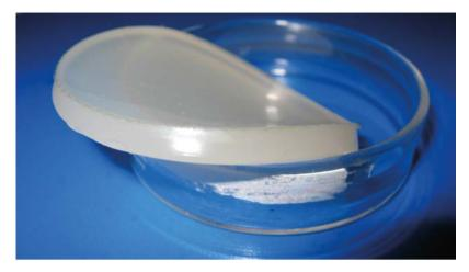
**Figure 3.23.** *Xylan-based hydrogel contains 90 per cent water, but remains mechanically quite durable. (Source: VTT)*
