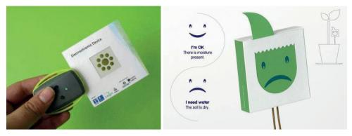
**Figure 3.17.** *Electrochromic Printed Electronics prototypes: free design for customised applications. (Source: CeNTI and Ynvisible)*
